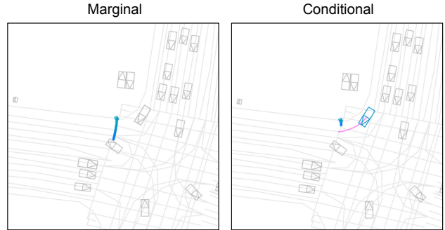
Figure 7. Visualization of the most likely predicted future for the pedestrian in the marginal setting (left) and temporally causal conditional setting (right). When considering the pedestrian independently, the model assigns greatest probability to a trajectory which crosses the road. When conditioned on the the vehicle’s ground truth turn (magenta), the pedestrian is instead predicted to yield.
