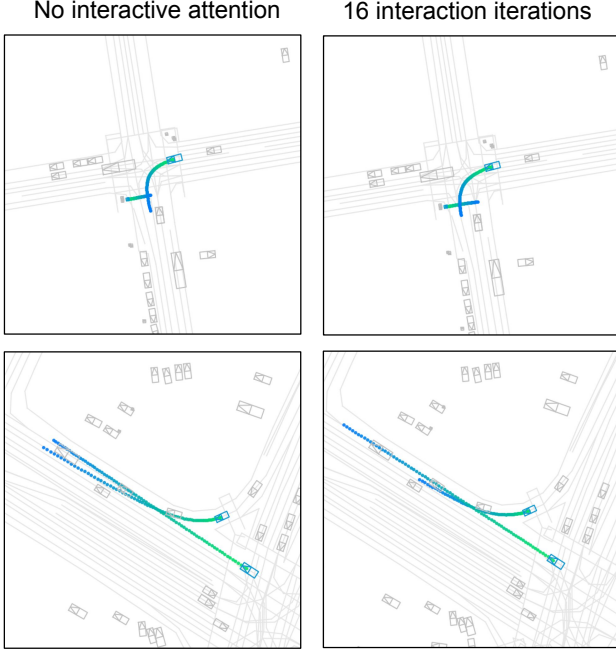
Figure 5. Visualization of the top joint rollout mode at the two extremes of the interactive attention frequencies studied here. With no interactive attention (left), the two modeled agents only attend to each other once at the beginning of the 8-second rollout and never again, in contrast to 16 total times for 2 Hz attention (right). The independent rollouts resulting from zero interactive attention can result in scene-inconsistent overlap; e.g., a turning vehicle fails to accommodate a crossing pedestrian (top left) or yield appropriately to a crossing vehicle (bottom left).
