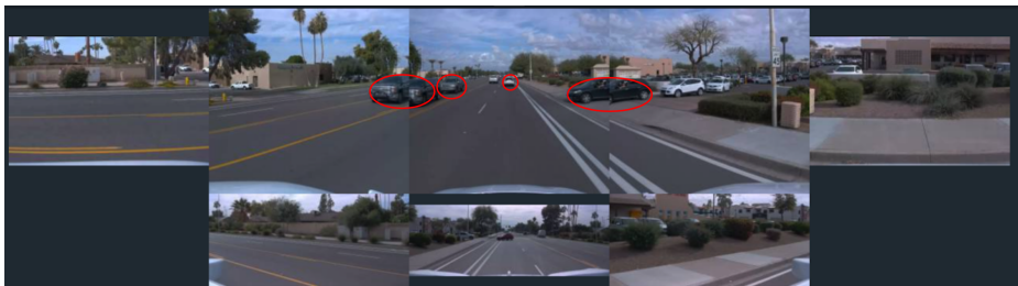
Fig. 2: Camera images from a randomly chosen scene in the labeling UI. The causal agents identified by the human labelers are circled in red.
